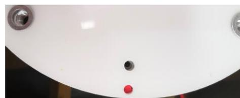
Figure 5 - Correct alignment is when the red dot is visible through the hole
