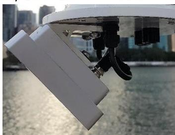
Figure 3 – Non-contact flow sensors
