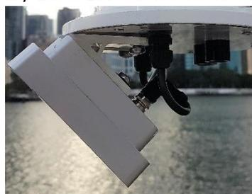
Figure 3 – Non-contact flow sensors
