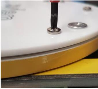
Figure 6 - Too much gap between plate and body
