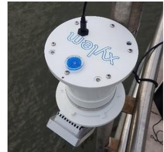
Figure 11 – Top mounted USB and bubble level
