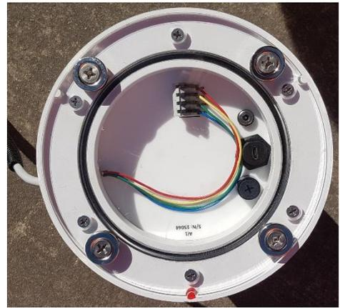
Figure 20 - Internal wiring for side gland entry
