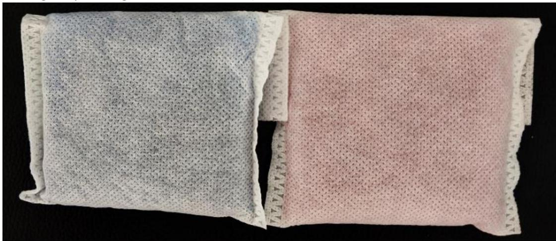
*Figure 24 – Fresh desiccant is blue (left). When orange (right) the desiccant must be replaced. Failure to use fresh desiccant will likely result in internal condensation and equipment failure.*
