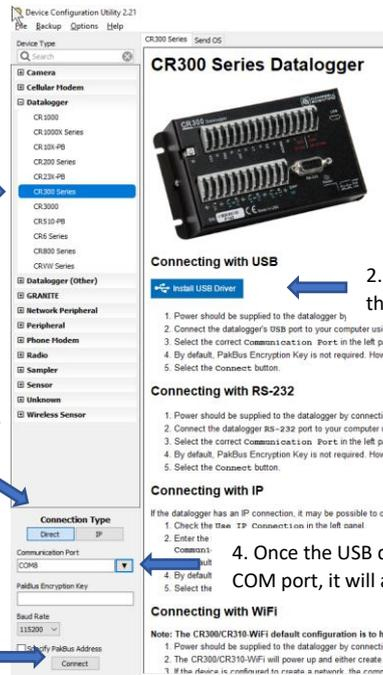
3. When plugging in a USB cable use the **Direct** type. If connecting through Eagle.io, use the **IP** type
