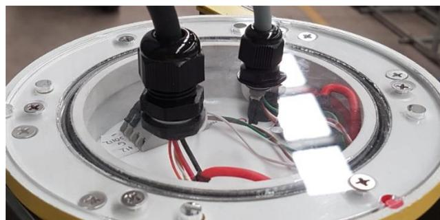
Figure 17 - Bottom plate fitted with M12 and M16 glands for waterproof cable entry
